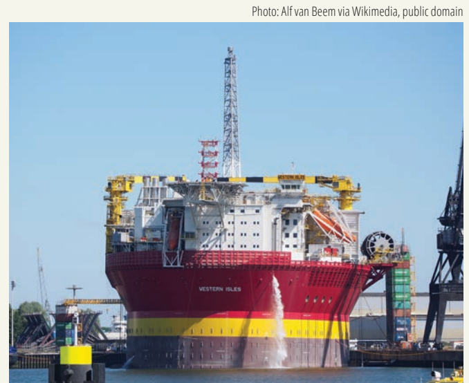
Floating production, storage and offloading vessels temporarily store oil at the offshore production site until it can be transported to shore by a barge or shuttle tanker.
