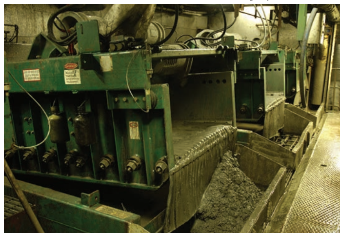
Shale shakers separate drilling mud from drill cuttings, which are one type of waste generated by offshore drilling that may be brought onshore for disposal.
